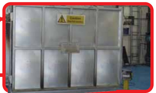
Firing Stage 2 The white is fired at 820 C in the furnace.
