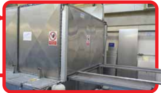
Degreasing A high quality detergent degreaser is used to remove surface impurities.
