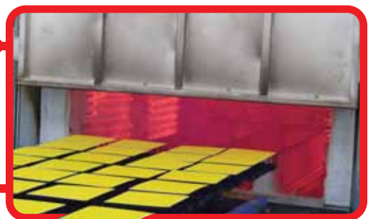
Final Print Firings Several firings take place at around 750C on multi colour signs.
