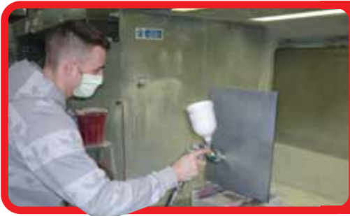
Top 'White' Coat The white or base colour coat is sprayed on to the grip coated surface.
