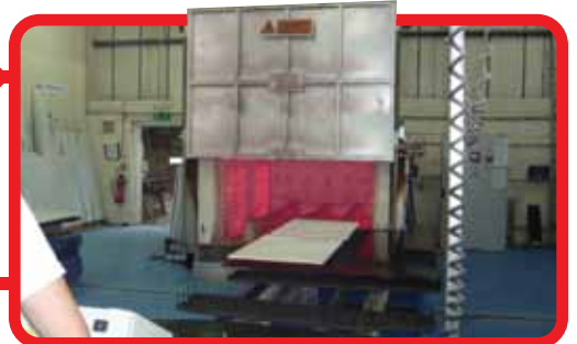
Firing Stage 1 The Grip coated steel is fired at a temperature of 860 C.
