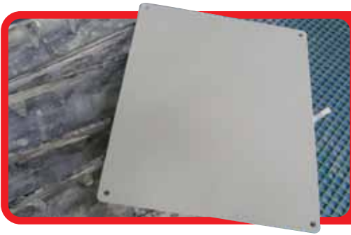
Base 'Grip' Coat Grip coat is sprayed evenly over all surfaces of the steel.
