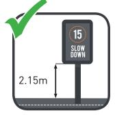
2.15m minimum between the base of the sign and the ground
